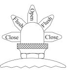
2. When the machinery has been standing idle for some time, hold toggle lever at a 45 degree angle for a short time. This will flush bearing and avoid dry start-ups.
