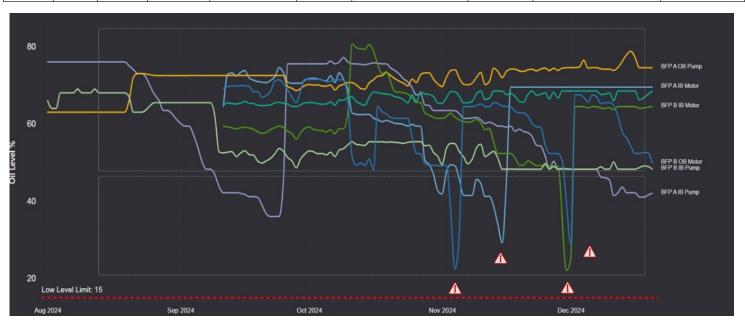
Low-level alerts detected a range of equipment-level events, including both sudden, event-based notifications indicating short-term lubricant losses and trend-based alerts revealing gradual lubricant depletion over a period of a month or more. These insights enabled proactive decision-making, allowing maintenance teams to allocate resources efficiently and address issues before they escalated, ensuring operational reliability and reducing downtime risk.
