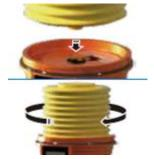
4. Refit the top housing on the lubricator. Turn the unit on and run test mode. Check to see if grease is dispensing.
